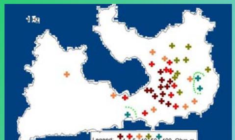
Figure 8. MT resistivity surveys: apparent resistivity map at 1Hz, which corresponds to electric current penetration down to 1000m.
