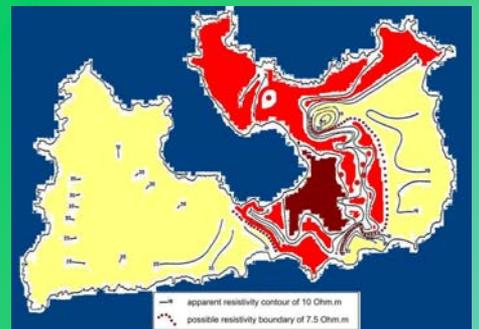
Figure 7. DC-Schlumberger resistivity survey: apparent resistivity map for AB/2 = 1000m, which corresponds to electric current penetration down to 700m.
