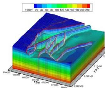
> 3D temperature distribution in the Basement and in the faults.
