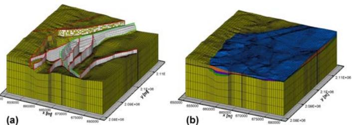
> Views of the Limagne Finite Element Mesh adapted from the geology model.
