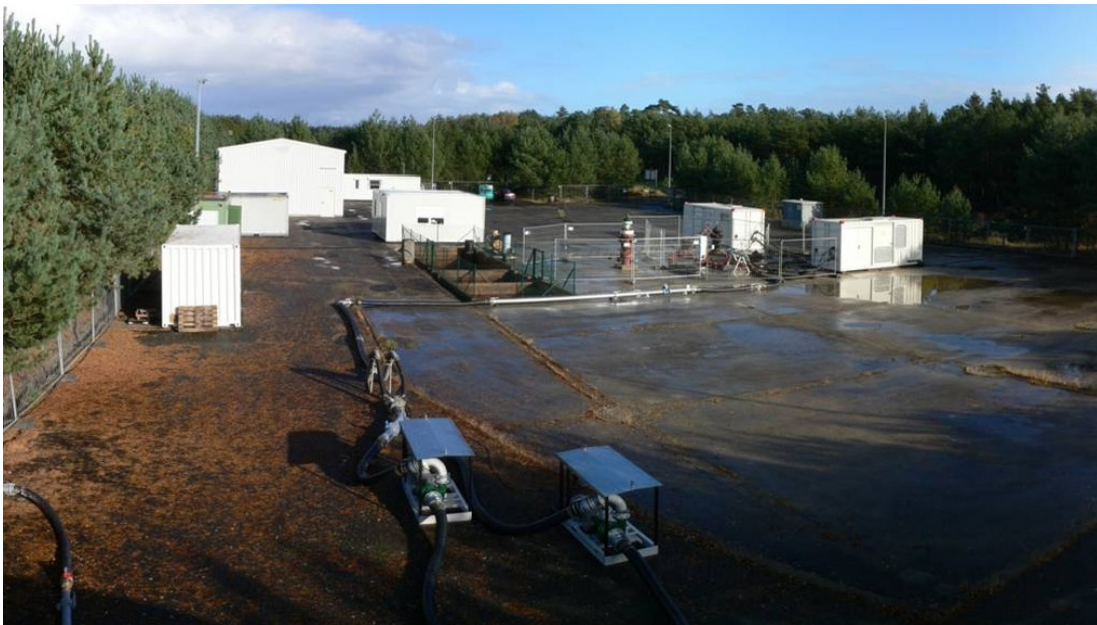
Figure 1 : Horstberg test site. The picture shows the setup of a hydraulic injection test using high pressure pumps.
