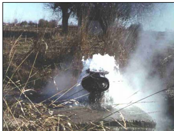
Fig.4: Artesian geothermal production well
