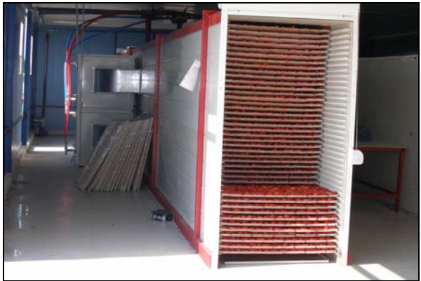
Fig.5: Geothermal dehydration tunnel loaded with tomatoes
