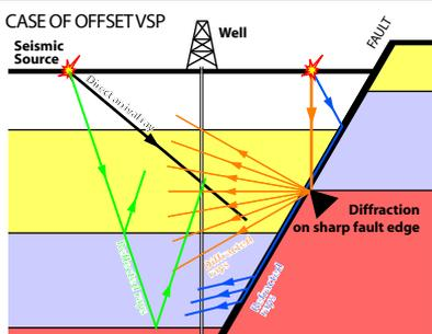
A Vertical Seismic Profiling is a field measurement procedure in which the seismic source is activated at a fix surface position and the seismic signal is recorded by sensors located in a well at successive depth levels.
