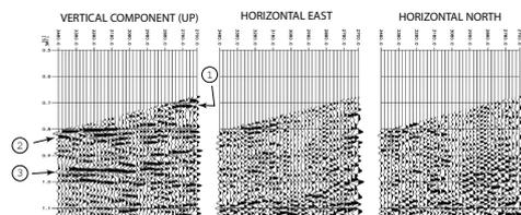
Most of the reflected energy appears on the VERTICAL component only, from dipping reflectors: it implies that the seismic reflections are recorded in SHEAR-wavemode by the VSP tool, after P-S conversion on the reflectors.
