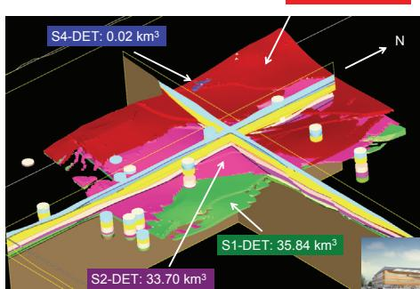
> The target geothermal reservoir corresponds to detritic rocks such as sand, sandstone and fluvial conglomerate because they have a higher probability of containing levels of permeable porous sandstones.
