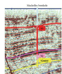
> Checking and fixing incoherencies. Seismic profile displaying spatial inconsistencies at Machelles borehole: S2MIXT surface has been set 100 m higher in the well than on the seismic profile and S2 surface 30 m lower.
