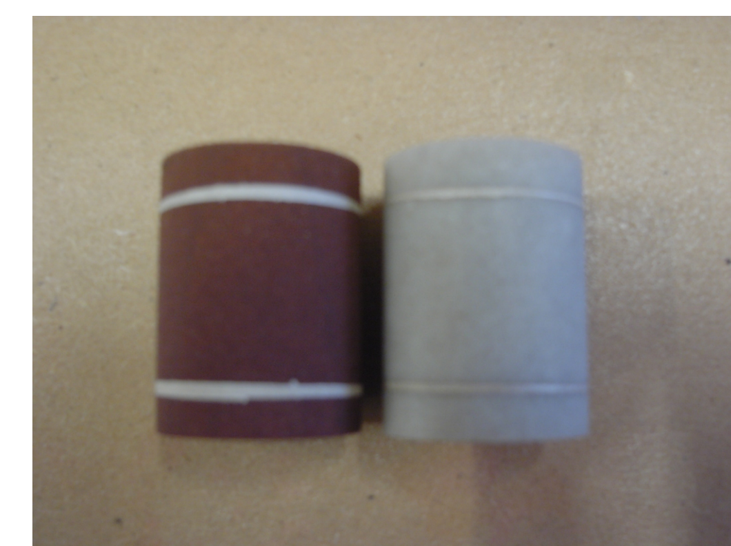
Fig. 5: Eberswalder Rotliegend (left) and Fontainebleau (right) samples with silver conductive paint rings for conductivity measurements. Sample size is 30 mm in diameter and 40 mm in length.
