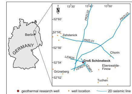
Figure 1. Location of the pre-existing 2D seismic sections and deep wells. The data were generated for gas exploration in East Germany.
