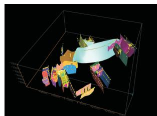
Figure 3. The fault model: Interpolation of grid nodes by inverse distance weighted average and minimum tension
