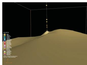
Figure 5. Bumps and dents: The result of non-statistical interpolation algorithms, in that well and seismic data have the same weights and are independent from distance and direction
