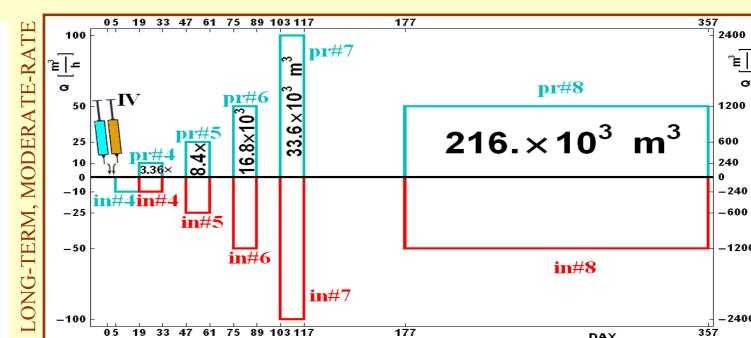
Our task: design and dimension 4 + 1 spikings at the boreholes GS4 + GS3 such that each individual spiking yields measurable signals during each of the subsequent outflow or abstraction phases (GS4 = new borehole, used for faulting, injectivity and sequential flow-back tests, 4 spikings; GS3 = old borehole, used for fluid disposal, i.e. reinjection, 1 spiking)
