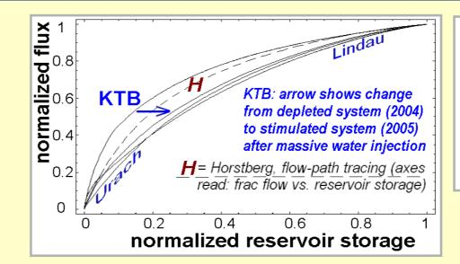
Flux-capacity analyses indicate what percentage of reservoir flow (if derived from flow-path tracings), or what percentage of solute or heat exchange (if derived from push-pull tests) takes place in a given fraction of the total reservoir storage, in the form of a cumulative repartition function, sorted by fluid residence times. This type of analysis (being well-known from reservoir hydraulics) was first applied for interpreting tracer tests in geothermal systems in the USA by Mike Shook (2003).
