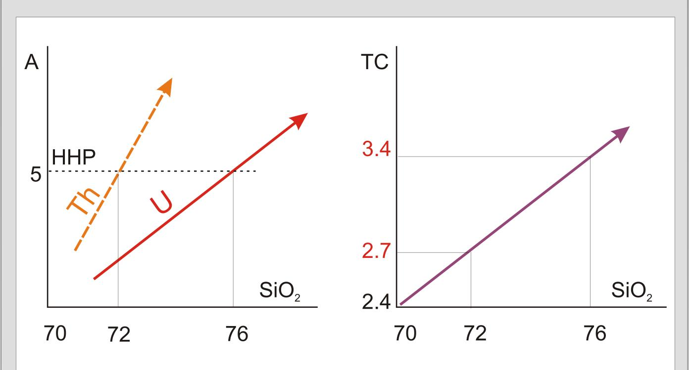
General trends of increase in radiogenic heat production (A) and thermal conductivity (TC) with increasing SiO<sub>2</sub>.
