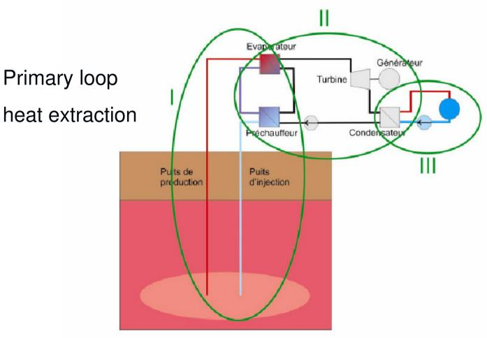
Cooling loop heat rejection
