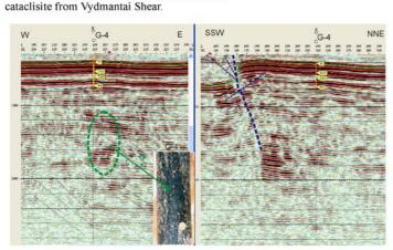
**Profiles E, G.** Crosses well G-4 at two different directions. They reveal reflection anisotropy. A strong reflection body is crossed that is traced from well G-2 to well G-4. Its nature remains uncertain, but those wells show specific high-angle
