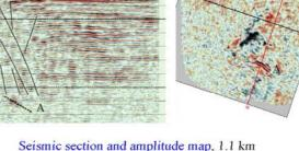
Seismic section and amplitude map, 1.1 km bellow the basement top. Telsiai fault is well identified. A strong reflector is traced at the depth 3.5 km that has similar features to low-
