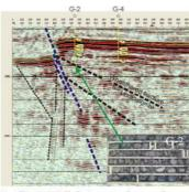
Profile B. Well G-2 crossed strongly fractured utramilonitic weathered zone at depth 2315 m (photo). It correlates with low angle reflector. A complex geometry of Telsiai fault is seen.
