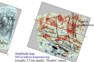
of Telsiai fault is recognised in the east (subvertical and inclined to the north features). Vydmantai shear is clear. Anisortopic fabric is evident to the west.
