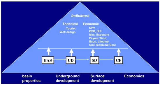
Fig. 1 fastmodel components for deep Geothermal systems.
