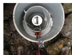
Installation and orientation of a Guralp seismometer CMG-40T (60 s) in a 1 m deep hole.
