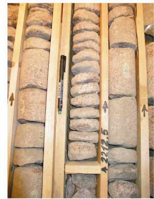
STRUCTURES IDENTIFIED IN ANOROGENIC GRANITOIDS UK - ultracataclasis, K - cataclasis, M - massive. Subhorizontal cataclasis is more common for the northern part of the intrusion.
