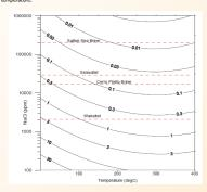
The resistivity of saline fluids shows experimentally a correlation with the temperature in the range 20-400 °C, as shown above. Although geothernal fluids contain a wide range of anions and cations, NaCl tends to be the dominant conductive species in the deeper parts of systems and other ions can be considered as Na or C appulaeties for the purpose of estimating resistivity. When Archies law is also applied, resistivity should vary with Temperature and processly following the graph shown below
