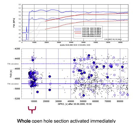
Failure pressure of all intersecting fractures
