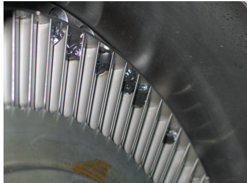
Pieces of rubber found in turbine
