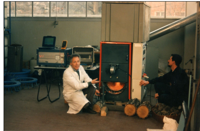
1987: A 3 kWel ORC turbogenerator biomass CHP plant in Milan
