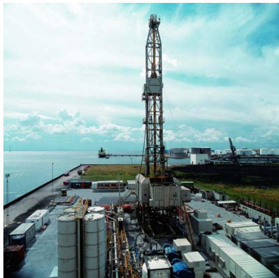
Fig. 3. The increasing involvement in geothermal related activities has so far resulted in two successful exploration wells near Copenhagen, Margretheholm -1 and -2.
