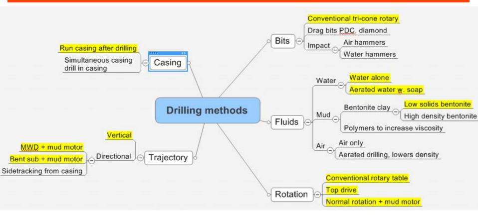
Various methods found in geothermal drilling. Yellow indicate the most common ones.
