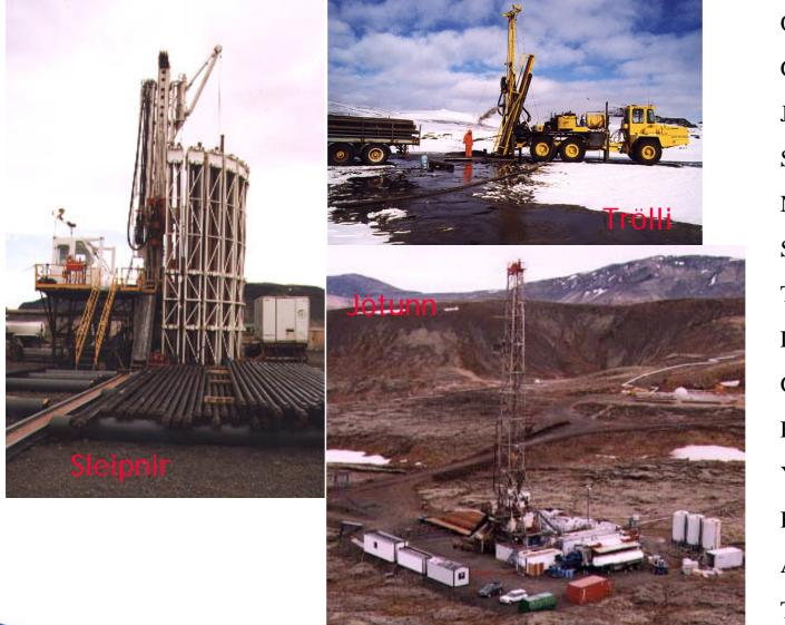
Óðinn JB 4000 m Geysir JB 4000 m Jötunn JB 3300 m Sleipnir JB 2400 m Nýr bor RFS 1600 m Saga JB 1350 m Trölli RFS 1100 m Langþr. RFS 600 m Glámur RFS 600 m Einráður RFS 500 m Ýmir JB 1000 m Hrímnir JB 300 m 300 m Alvarr **Trítill RFS** 120 m
