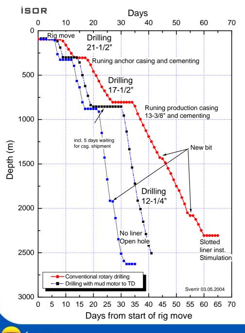
Drilling progress – days vs. depth
