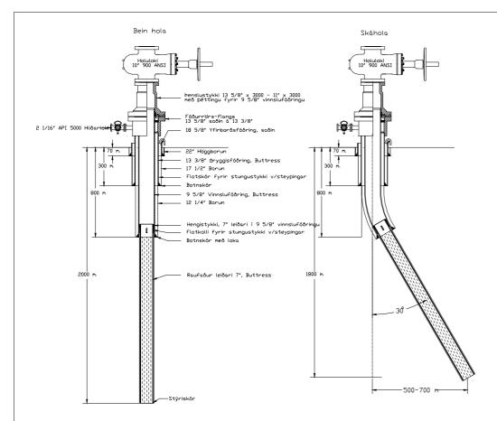
The casing programmes are virtually the same. The build-up starts at the kick off point (KOP) at 300-500 m.
