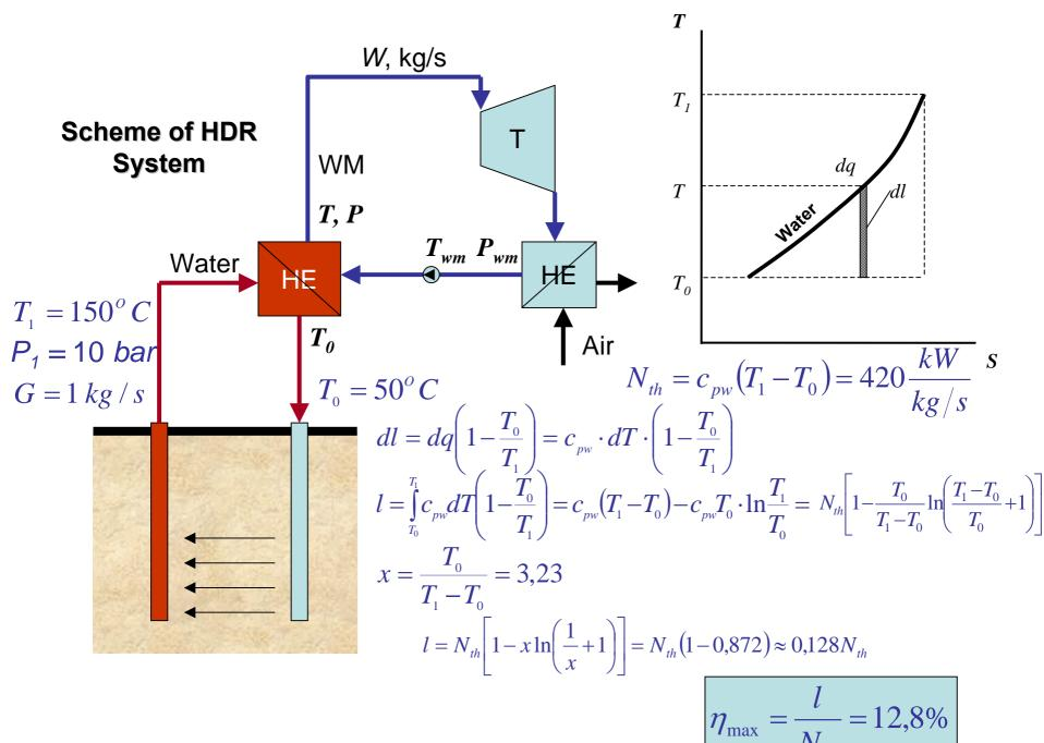
The thermal power of the water flow is transmitted to a working media (WM).
